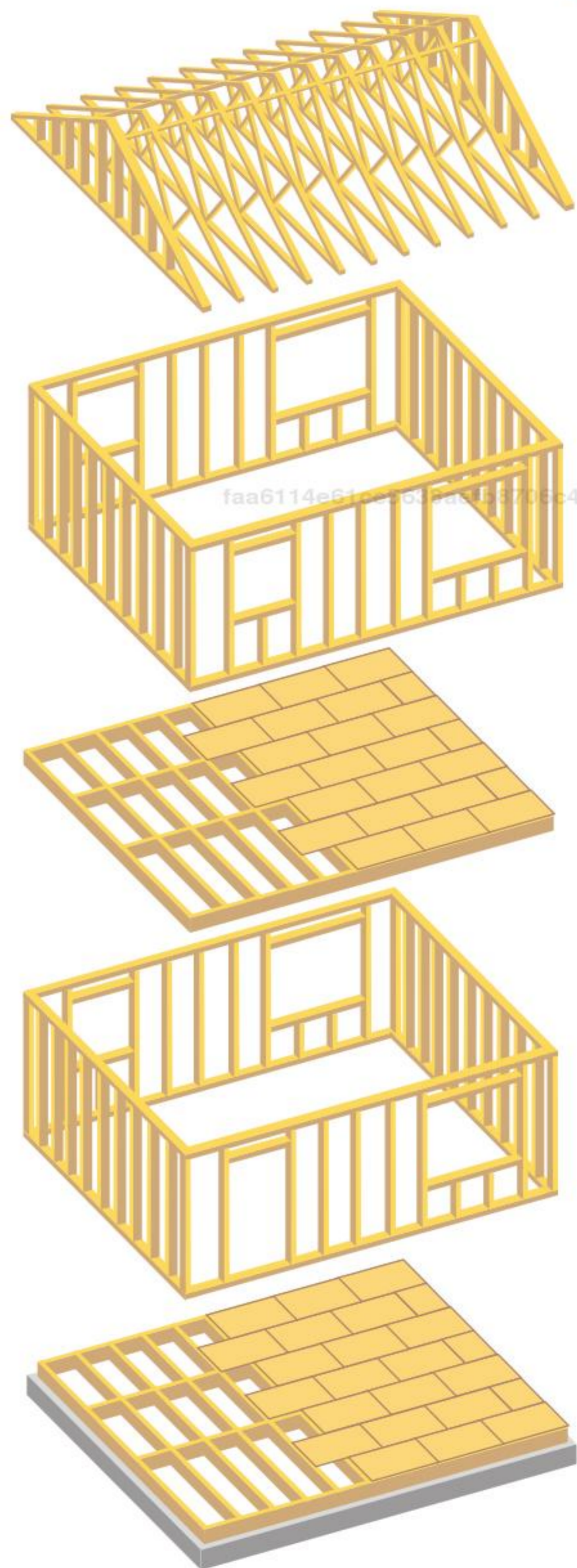
▲ Figure 6.5 A timber-framed house
