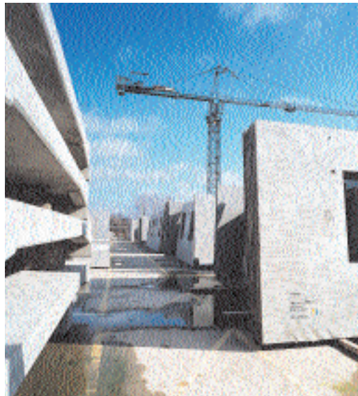
Left: Typical wall units in manufacturer's stockyard (courtesy of Tarmac Precast Concrete Ltd)
