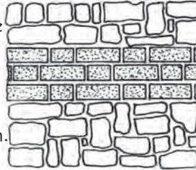
Random rubble with brick lacing
