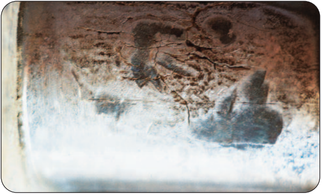
Figure 32 - Mode of Failure - Impact & alignment
