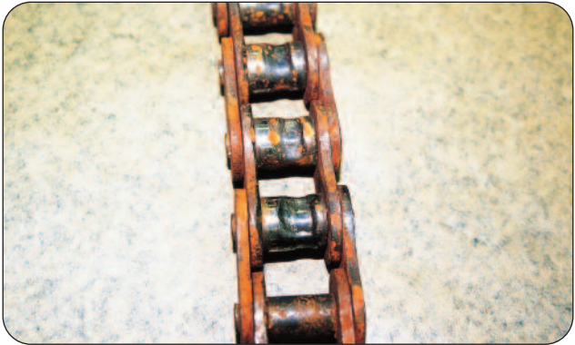
Figure 4 - Mode of Failure - Corrosion
