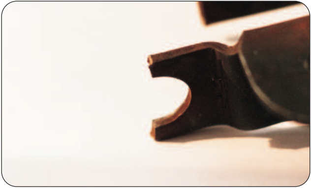
Figure 43 - Mode of Failure - Tensile overload
