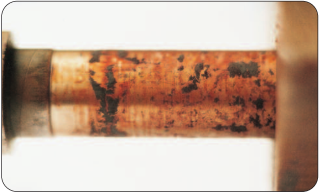
Figure 31 - Mode of Failure - Fretting
