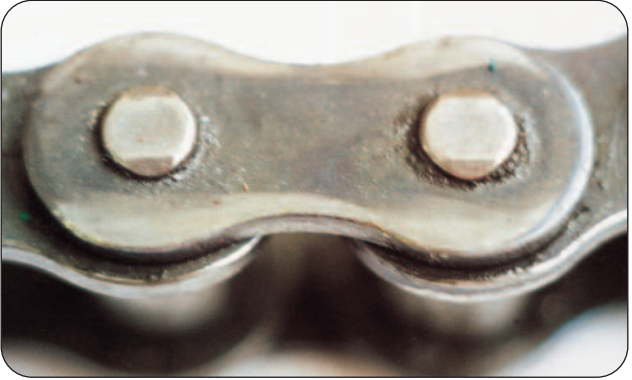
Figure 1 - Mode of Failure - Alignment
