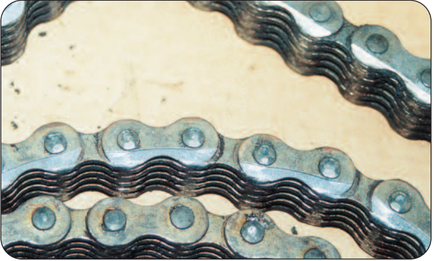
Figure 45 - Mode of Failure - Alignment
