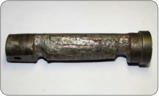
Figure 7 - Mode of Failure - Erosion
