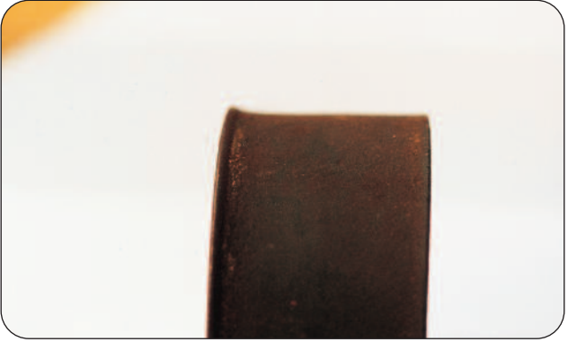
Figure 34 - Mode of Failure - Misalignment
