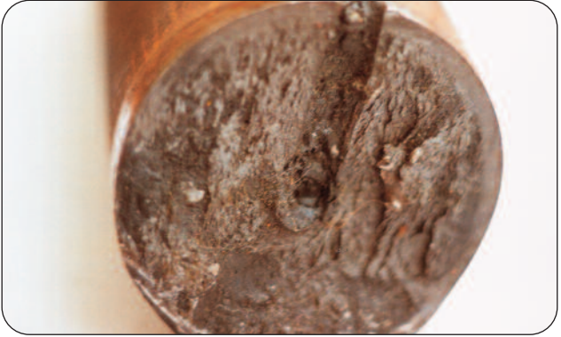
Figure 35 - Mode of Failure - Misalignment
