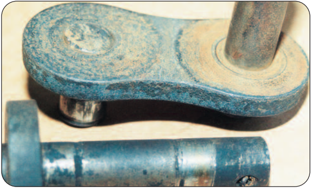
Figure 16 - Mode of Failure - Lubrication & Alignment
