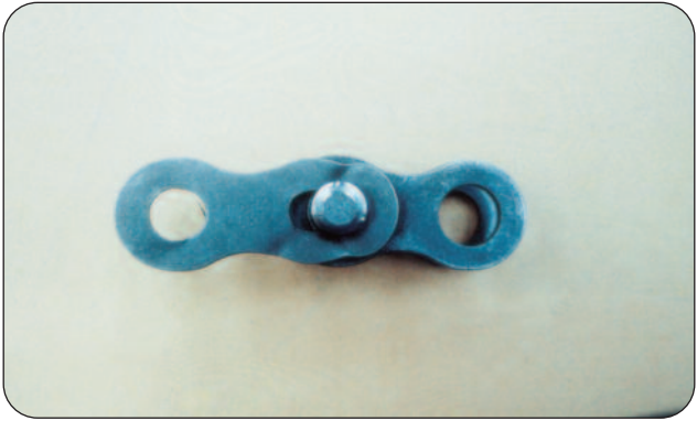
Figure 18 - Mode of Failure - Overload
