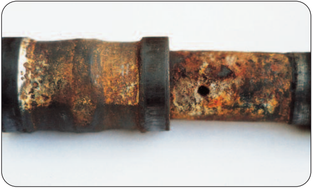
Figure 29 - Mode of Failure - Corrosion/Erosion
