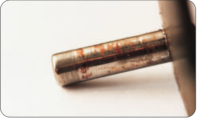
Figure 11 - Mode of Failure - Fretting Corrosion
