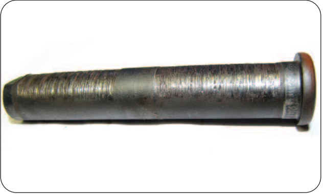
Figure 13 - Mode of Failure - Galling
