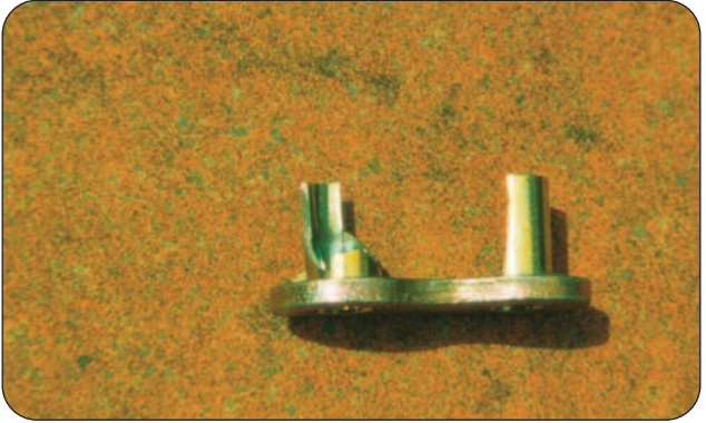
Figure 9 - Mode of Failure - Fracture
