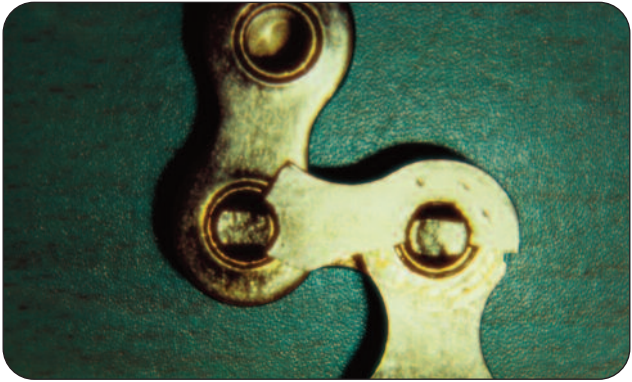
Figure 10 - Mode of Failure - Fracture
