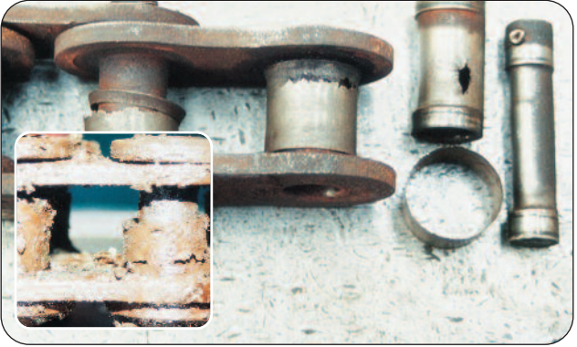
Figure 3 - Mode of Failure - Corrosion
