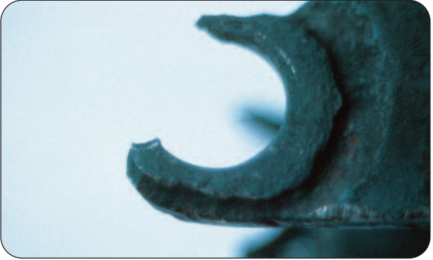
Figure 30 - Mode of Failure - Corrosion/Erosion
