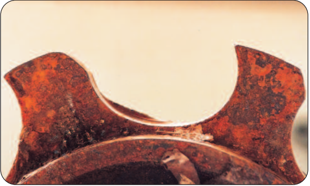
Figure 26 - Mode of Failure - Alignment
