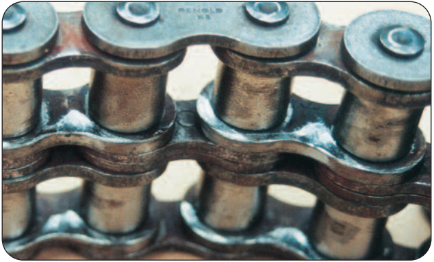
Figure 14 - Mode of Failure - Lubrication & Alignment
