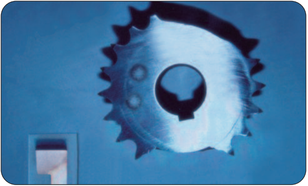
Figure 17 - Mode of Failure - Material cracking below teeth
