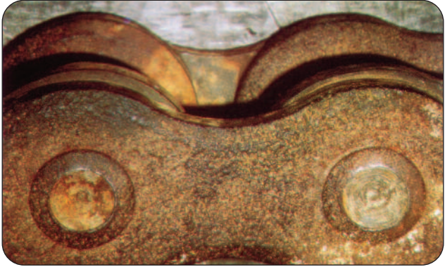
Figure 20 - Mode of Failure - Pitting Corrosion
