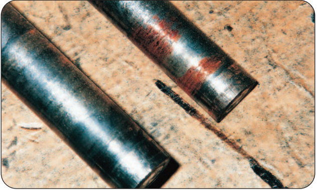
Figure 47 - Mode of Failure - Galling & fretting corrosion
