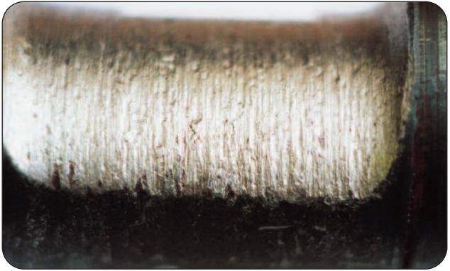
Figure 37 - Mode of Failure - Overheating
