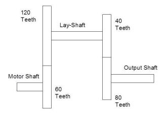
f) The sketch shows the compound drive train for a lathe headstock, calculate the output shaft speed if the motor shaft speed is 3000 RPM
