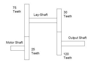
g) The drawing shows a compound gear arrangement on a bench drill. Calculate the output spindle shaft speed if the motor speed is 1500 RPM.
