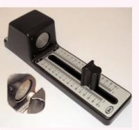
counter with a 4 cm diameter window and a vertical array of 17 wires. A standard cup-type alpha-emitting radioactive source and a school 5 kV EHT power supply are also needed to make it work, and rapid sparks can be counted by connecting a scaler (digital counter). The IPC spark counter is available for around £175 from: Scientific and Chemical
