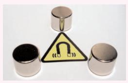
Where extremely high magnetic fields are required, small magnets made from rare earth elements can be used. These are made from sintered, compressed powders, which often contain neodymium, iron and
