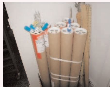
The strong cardboard cylinders in which burettes are delivered can be secured in a quiet corner and used as a burette store. Try to stock up with 25 cm 3 burettes, which are more easily filled than standard 50 cm 3 versions.
