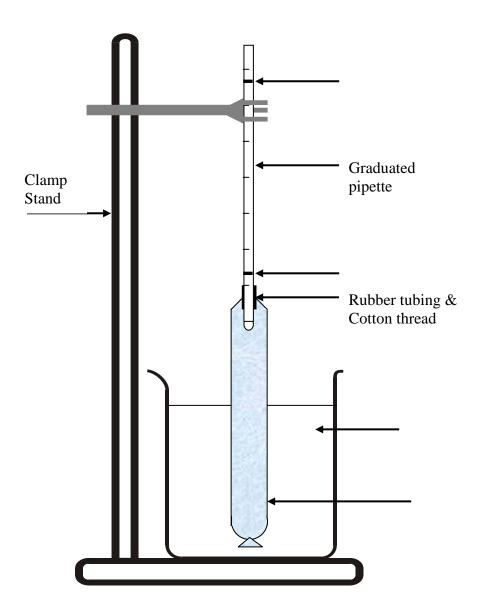
Add the following labels to your diagram:Sugar solution, water, semi permeable membrane, initial level, final level.
