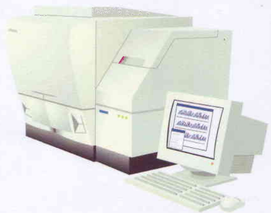
▲ Automated sequencing machines are able to determine 450 000 bases per day. The interpretation of the vast amount of sequence data produced means that bioinformatics is of increasing importance.
