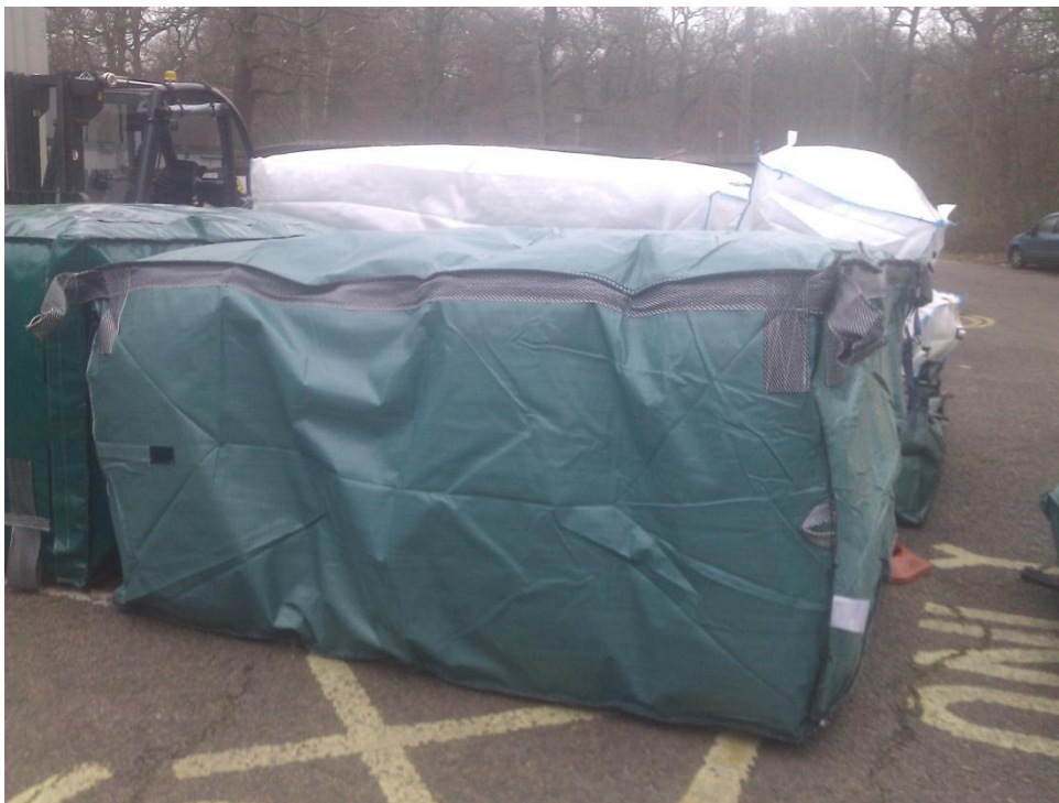
Photo: Fall & arrest bags for testing (Courtesy of BRE)
