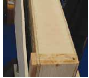
SIP panel showing construction
