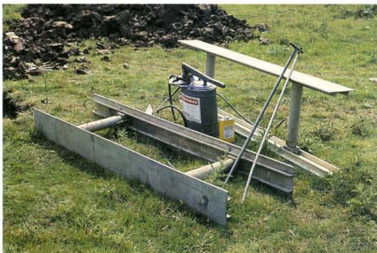
Fig 3 Hydraulic trench shores and hand-operated hydraulic pump; the lowering handles also operate the pressure release valves
